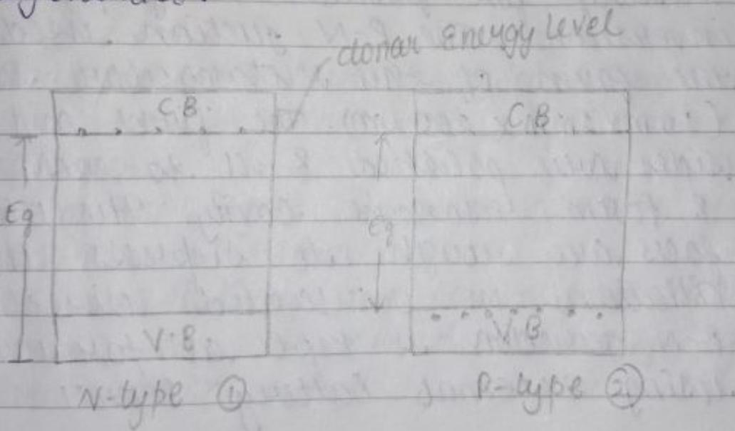
In fig (2) the acceptor energy level is just above the top of V.B. at  $\Delta E = 0.01 \text{ eV}$ . When temp. of p-type semiconductor is gradually increased from 0K, the transition of  $e^-$  from V.B. to acceptor energy level takes place around 20 to 50K, the acceptor energy level will be completely filled &  $e^-$  raised to this level leaves behind holes in V.B. This makes the material
